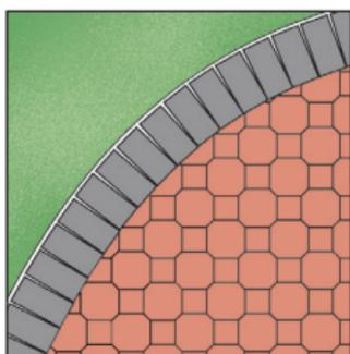
Add a professional touch to your pavement by using Boston or Georgetown Colonial Pavers® as a soldier or sailor course along the outside edges to finish the border. This technique works well with almost any style of paver and pavement shape, including curves, by “framing” the pavement for a neat finished appearance. See page 17 for more information on soldier and sailor border courses.
