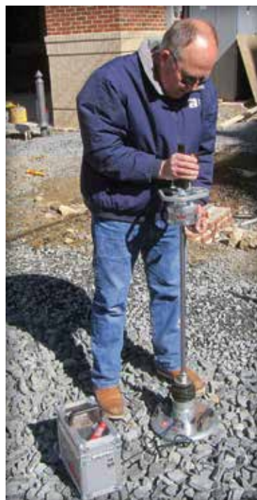
Figure 22. Testing base stiffness using light-weight deflectometer.
