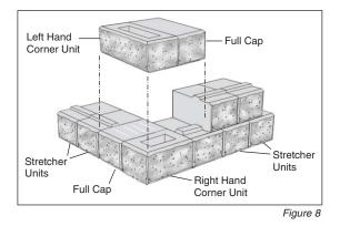
As you lay out the location of the wall, mark the position of the corner with a stake and use string lines to indicate the line of the intersecting walls. When digging the trench, allow for additional space at the corner location.
