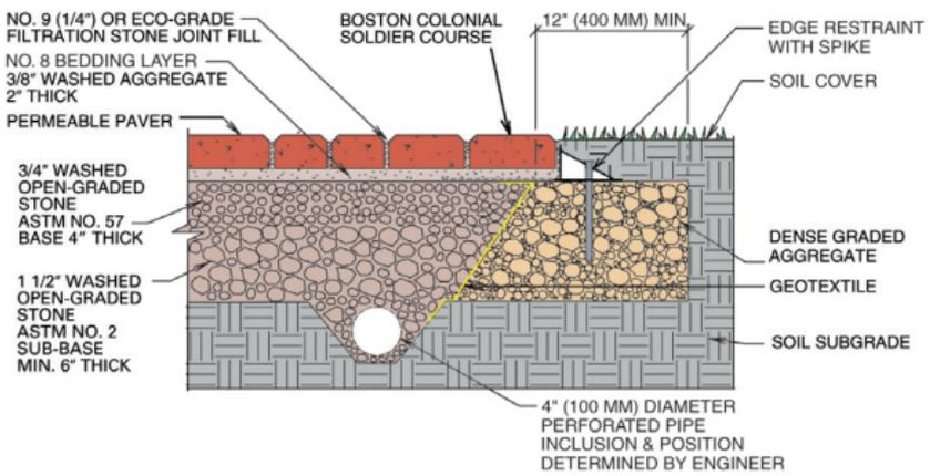
**Edge Restraint** - Holding permeable pavers in place is as important as it is for our regular pavers. You will need to install edging along the perimeter wherever there is an unrestrained edge. Driving spikes into a graded stone base can be difficult, so we suggest using one of two options.
