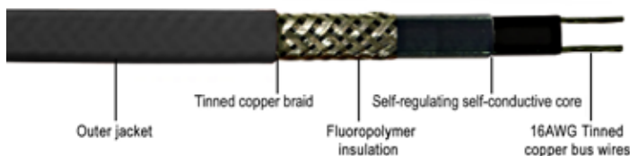
ProLine (PLSRS) self-regulating pipe trace cable.
