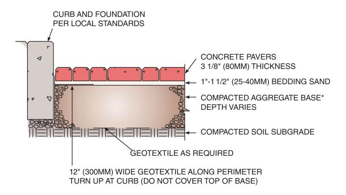
\*Base may also be asphalt, concrete or flowable fill
